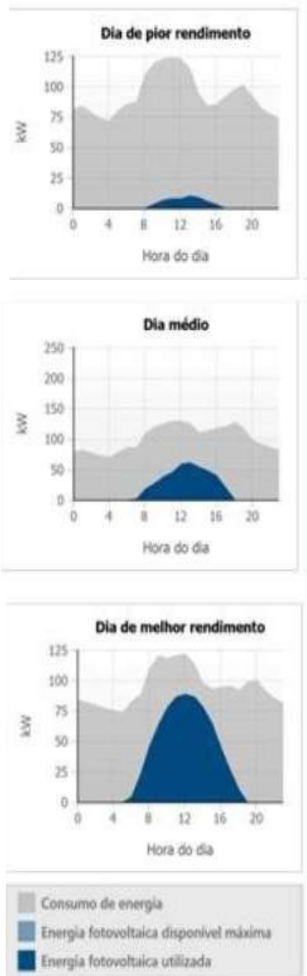
Figure 1. Estimates of PV energy produced (SMA Simulator)
