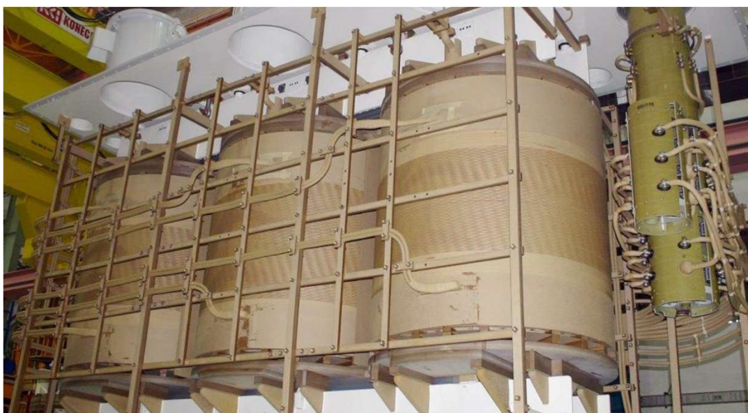
Figure 3 - Transformer active part isolated with Kraft paper
