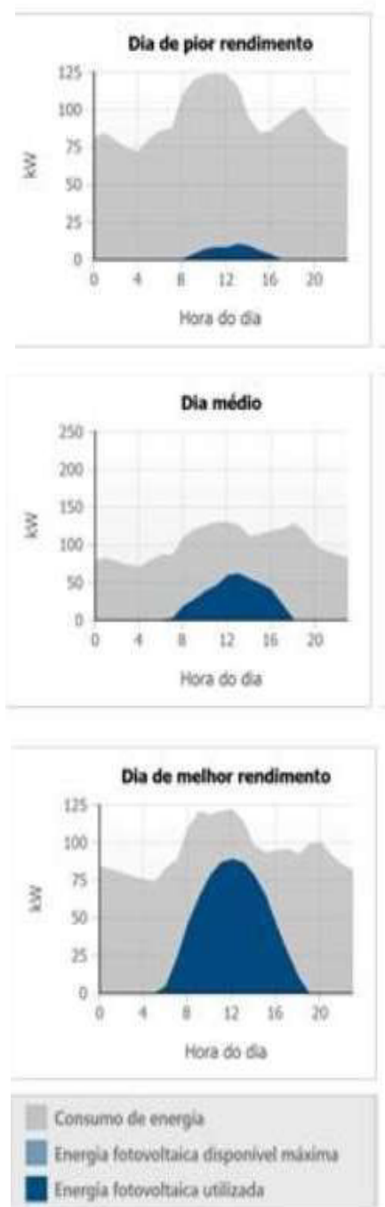
Figure 1. Estimates of PV energy produced (SMA Simulator)
