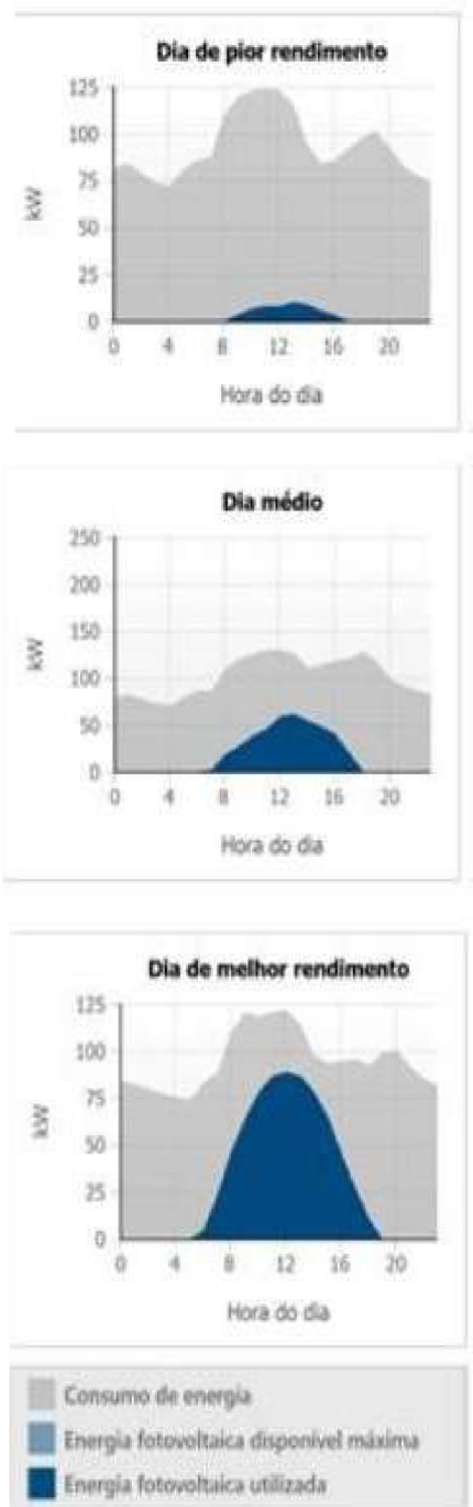
Figure 1. Estimates of PV energy produced (SMA Simulator)
