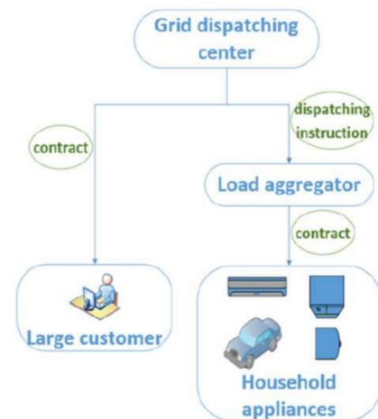
Fig. 4. Relation between the user, load aggregator, and the grid dispatching center [16]
