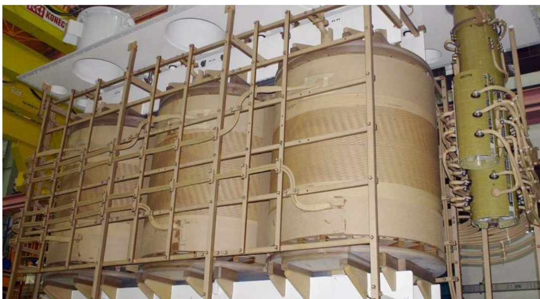
Figure 3 - Transformer active part isolated with Kraft paper
