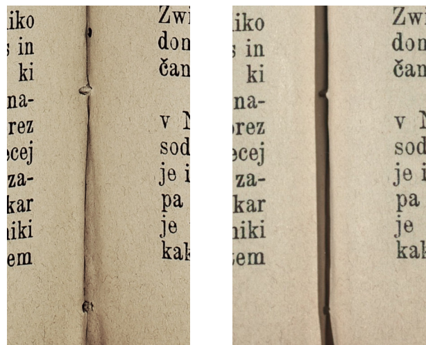
Figure 2. The same part of the book digitized left without glass and right with glass. There is an obvious difference in the amount of useful detail on the page link. On the left we see that, for its protection, the book is not opened 180 degrees, which is not the case on the right.
